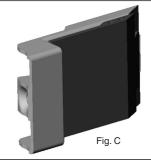
To fasten the oven to the cabinet, open the door of the oven and attach it by inserting the 4 screws (supplied with the appliance) into the 4 holes located on the perimeter of the frame.
